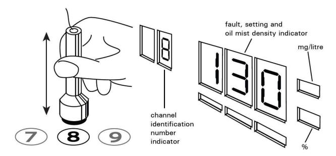
Once the key has been turned, the channel adjusted should go straight into main alarm. Please then reset the alarm level and then reset monitor using the magnetic pen on the reset button. The engine shut down will also need to be reset, if used and the engine restarted and checked for correct operation.
