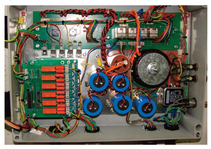
This was used for several different variations of the Multiplex from the earliest models (these have 12 plugs installed into the bottom of the panel and no junction box up to the Harting connectors). The image above shows a Monitor PCB with Individual shutdown 2 x 6.
