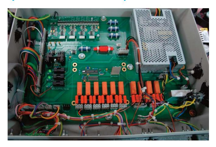
This is the third generation board and the latest version of the system, running in conjunction with the new MP12 processor board. The image shows a board with data logging and 2 x 6 individual shutdown installed on it.
