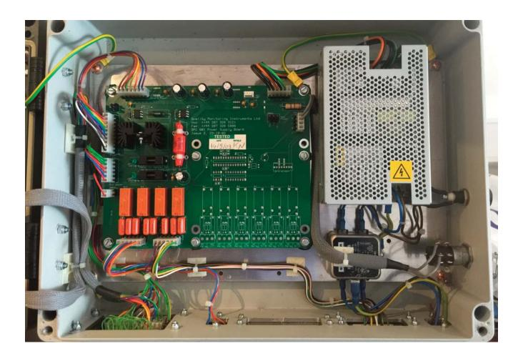
This is the second version of the relay board and power supply with solid state relays, separate power supply bolted to an aluminium plate. This board will only come with Harting connectors (unless upgraded from previous state).
