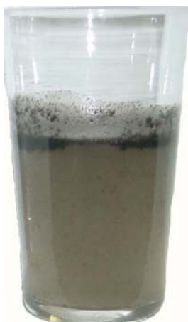
Influent Bilge Water inc, free Oil and Emulsions
